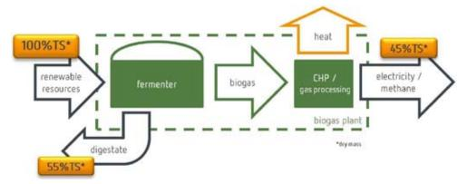
Biogas plants combined with maxbiogas LX-plants convert 95% dry-matter of the same substrates to biogas and also separate only the compounds which are responsible for fertilisation.
